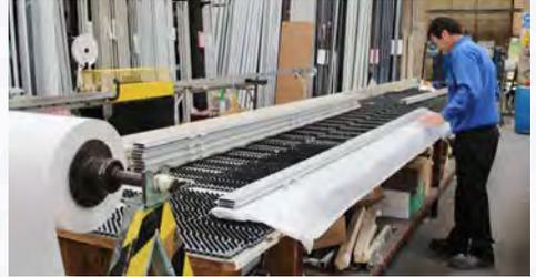
Using fully automated spiral wrappers material is securely packed, this also gives a durable clear protective coating to all bundles.
