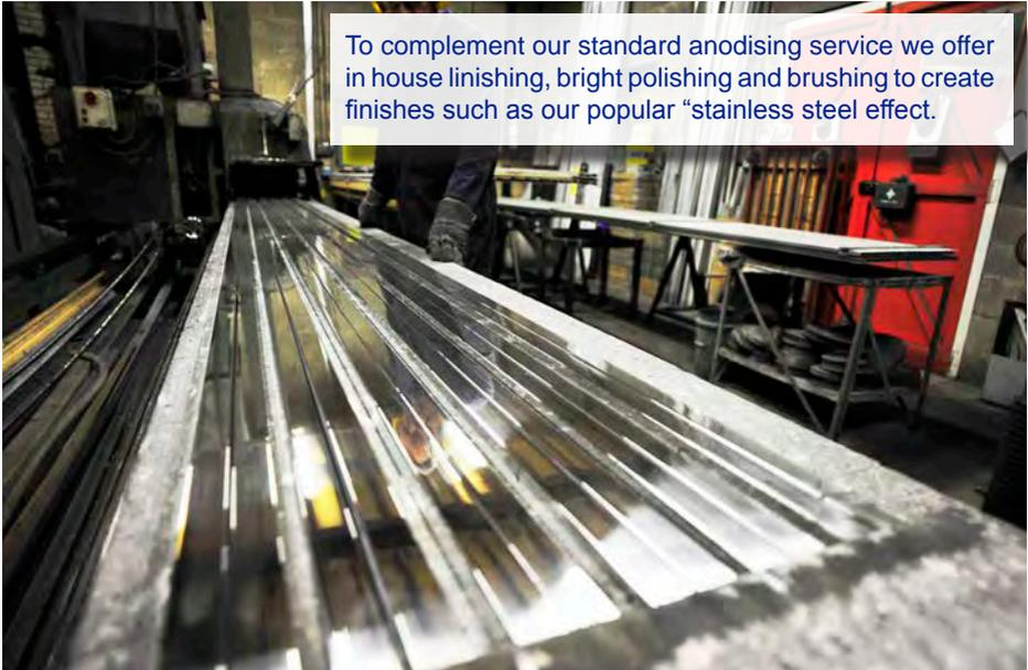
Using a variety of chemical and mechanical techniques prior to anodising we can radically affect the final appearance of aluminium. The resulting finish is UV stable, weatherproof and hard wearing.
